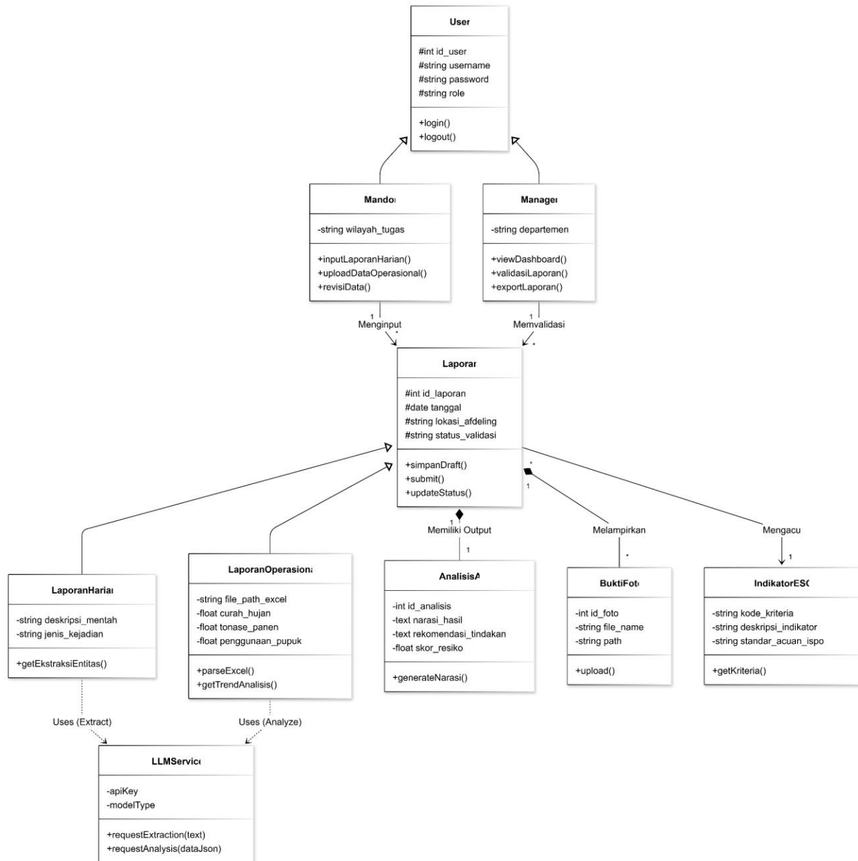
Figure 1. Class diagram of the proposed MVC-based system architecture
