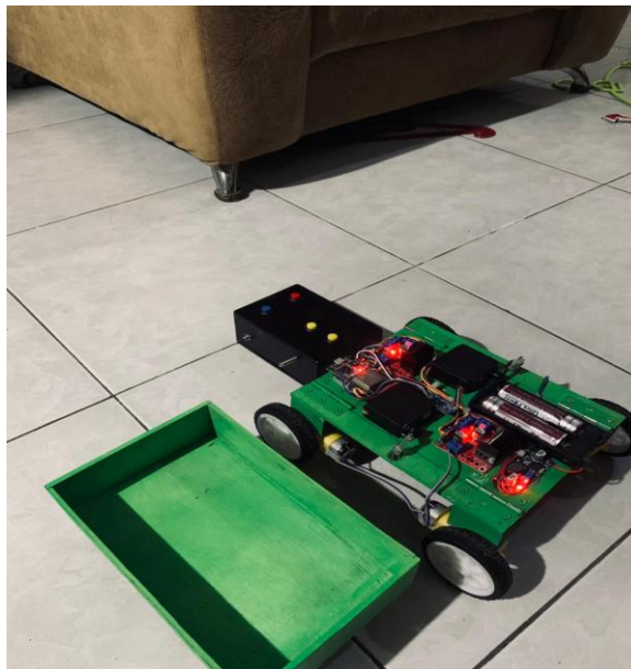
Figure 2. Developed Motor-Balancing Prototype for Fresh Fruit Bunch Transportation
