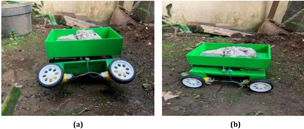
Figure 5. Wheel Mode Performance Testing: (a) crawler mode on simulated muddy terrain; (b) loader mode on simulated rough terrain
